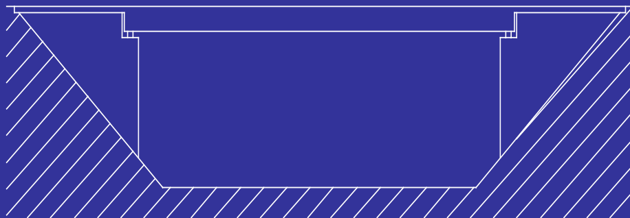
Extended Deck Bridge
